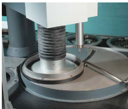
4. Grinding is now in operation. The next specimen holders are ready for collection
