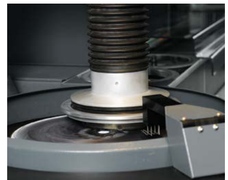
6. After fine grinding the specimen holder moves on to polishing
