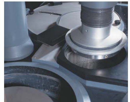
5. When the grinding is completed, the specimen holder is carried to the cleaning chamber
